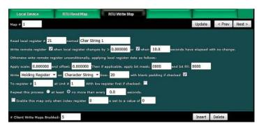
Interface to a Modbus RTU alphanumeric display device has never been easier. The SPX Pro-V2 recognizes a series of Modbus holding registers as a single character string. The built-in Script Basic includes richly featured character string manipulation and recognizes the series of registers as a single character string.
