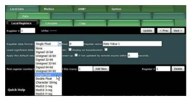
Configuration of the gateway is done via the web pages served by the internal web server. The user simply fills in templates. The entire configuration is saved in the internal Flash file system in XML format. This file may be exported to replicate additional copies of the configured device, or for backup.
