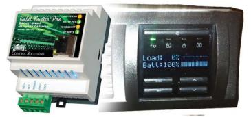
The alarm table in a typical UPS system cannot be directly polled due to the fact that alarm table entries are only present while alarms are present, and attempts to poll the alarm data with no alarms present will result in errors. The table walker in the Pro-V230 has the intelligence to scan the alarm table for alarms, and set BACnet Binary objects to Active when alarms are found, and automatically clear Binary objects to Inactive after a timeout when not found.
