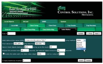
Configuration of the gateway is done via the web pages served by the internal web server. The user simply fills in templates. The entire configuration is saved in the internal Flash file system in XML format. This file may be exported to replicate additional copies of the configured device, or for backup.
