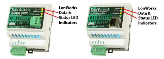
The LonWorks indicator LEDs display LonWorks network activity. Note, however, that activity of these LEDs is not only affected by configuration of the device, but by whether the device is commissioned on the network and whether other devices are also communicating.
