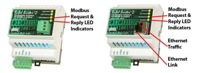
The request and reply LEDs will indicate Modbus traffic as indicated in the table below.
