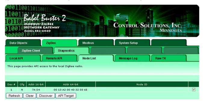
When a device is first connected, it will hopefully show up in the Node List. For this to happen, it must be configured with the same stack profile as the BB2-6040 (ZS parameter), and must be set for the same PAN ID, or set to "join any" PAN. Devices configured to use AT mode instead of API mode will also not show up here, but that does not mean you cannot communicate with them. Check the Message Log page to see if your device is sending anything the BB2-6040 can hear.
