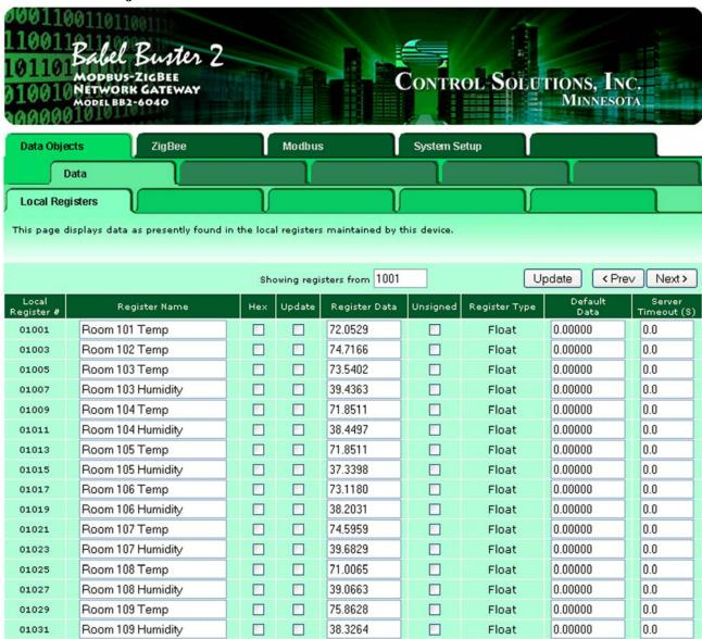
The contents of the set of local registers found within the BB2-6040 is displayed here. You have the option of forcing a new value by entering a value, checking the Update box, and clicking Update. If hexadecimal display format is more useful for packed 16-bit registers, check the Hex box. The Unsigned check box simple applies to how the data is formatted when displayed on this page.
