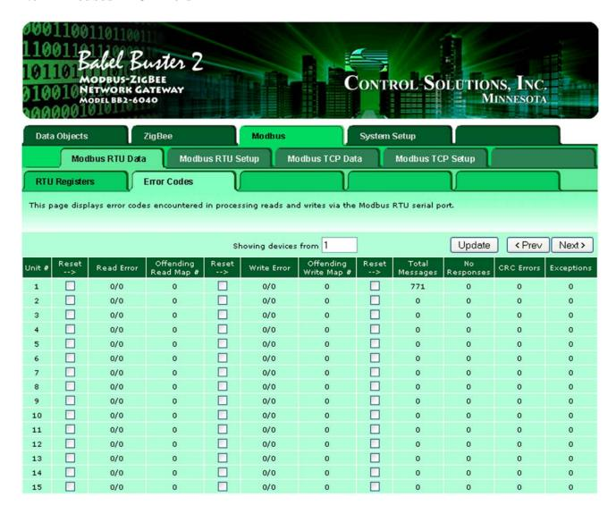
The first occurrence of read and write errors are shown along with the map number that was being processed when the error occurred. Check the reset box and click update to clear it and possibly show the next error if there are more than one active error conditions.
