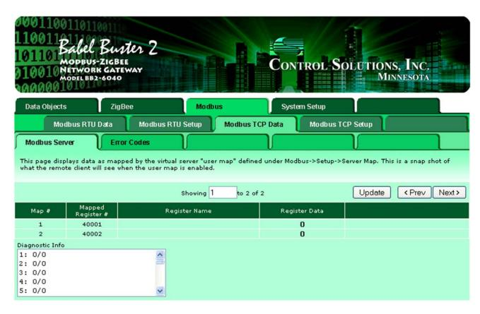
The values of Modbus registers that have been created by the virtual server mapping are displayed on this page. These are the values that a remote client would see. (The remote client acts as Modbus master, and this server acts as a Modbus slave having the registers shown here.)
