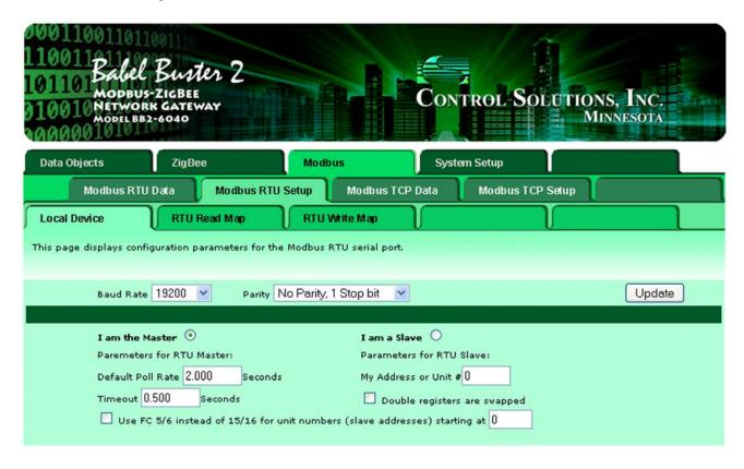
Select baud rate and parity from the drop down list. Click either Master or Slave buttons to select type of operation. Enter timing parameters or address as applicable. Click update to register your changes.
