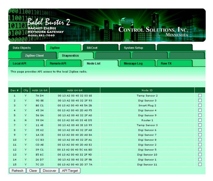
This page shows the list of devices that have associated themselves with the BB2-6040's ZigBee radio functioning as a coordinator. Click Discover to send the /ND command to the local radio. It will respond by sending its list of devices which are then displayed here. Click Refresh after waiting a short time for all of the responses. Click Clear to clear the page and repopulate the list.
