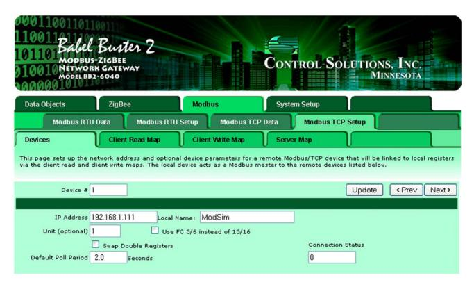
The Modbus Devices page is illustrated above. Device number simply shows you where you are on the device list. Click "next" and "prev" to scroll through the list.
