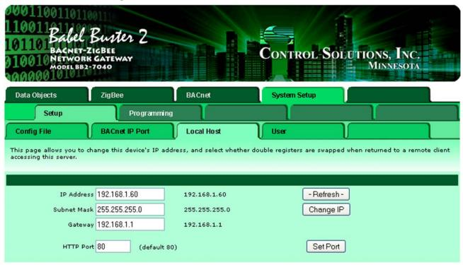
To change the IP address of this device, enter the address, subnet mask, and gateway, then click "change IP". Set the IP address to 255.255.255.255 to specify that DHCP should be used to obtain an IP address upon power-up. IP address change will take effect upon next power cycle.
