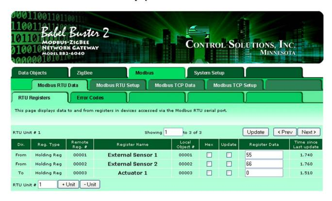
The values of Modbus registers that have been read from remote RTU serial devices is displayed here. One remote unit at a time is displayed. To display a different unit, change the RTU Unit #.
