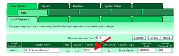
Error code registers are automatically named **-Sys Error**, **Fn #n** for system errors, **-TCP error**, **device #n** for TCP device errors, and **-RTU error**, **device #n** for Modbus RTU errors or BACnet device errors. In each instance of "device", the "n" is device number as referenced on other pages.
