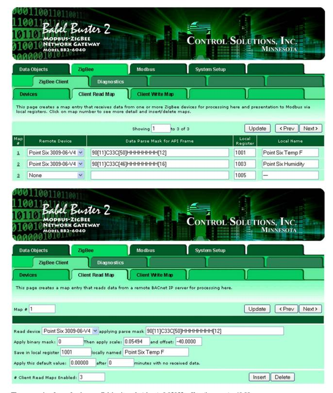
The conversion factor for degrees Celsius is scale (slope): 0.03053, offset (intercept): -40.00.
