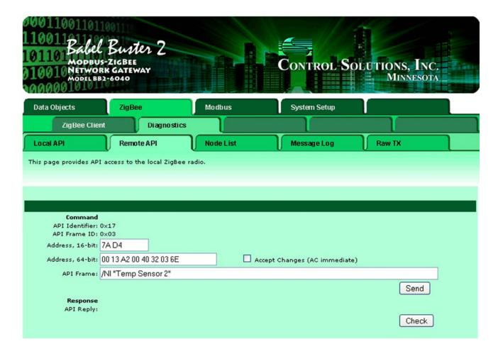
One of several commands you will send to a remote device, assuming it recognizes remote API commands, will be the NI or Network Identifier command. This assigns a name to this device, and after the WR command is sent, it becomes stored in the remote ZigBee device's non-volatile memory.
