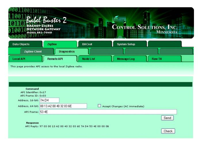
Remote API commands are constructed and sent on this page. Remote API commands work exactly like local API commands, except that they are sent to a remote ZigBee device. These API commands are specific to XBee PRO/Ember 250. Commands sent to ZigBee devices using a stack other than Ember will require construction of raw packets on the Raw Tx page.
