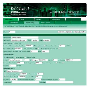
Pre-configuration of the gateway is done via the web pages served by the internal web server. The user simply fills in templates. The entire configuration is saved in the internal Flash file system in XML format. This file may be exported to upload to the web portal. Once the BB2-6010-Web is online "live", configuration is done remotely via the web portal.
