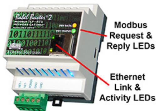
Babel Buster BB2-6010-Web request/reply LEDs reflect RTU traffic while the Ethernet activity LED will indicate TCP traffic. To see TCP errors, one needs to look at the Errors page in the web UI. (Note: If Modbus RTU is not configured for any use, then the request/reply LEDs will reflect TCP traffic; however, normally the only indication of TCP traffic is the Ethernet activity LEDs.)
