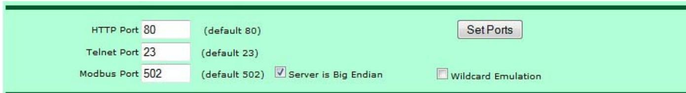
The screenshot shows a configuration interface with a light blue background. It contains three input fields for ports: HTTP Port (80), Telnet Port (23), and Modbus Port (502). Each field has its default value in parentheses. To the right of the Modbus Port field is a checked checkbox for "Server is Big Endian" and an unchecked checkbox for "Wildcard Emulation". A "Set Ports" button is located to the right of the top two fields.
