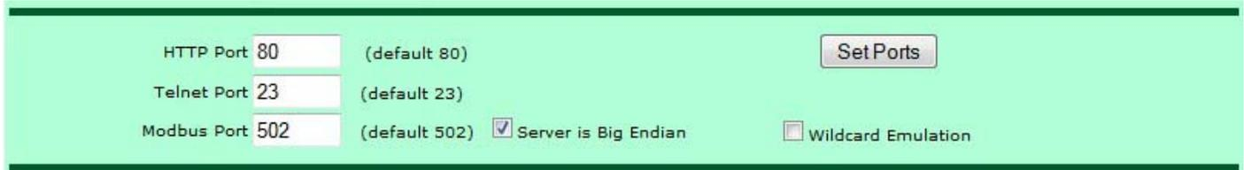
The screenshot shows a configuration panel with a light blue background. It contains three input fields for ports: HTTP Port (80), Telnet Port (23), and Modbus Port (502). Each field has its default value in parentheses. To the right of the Modbus Port field is a checked checkbox labeled 'Server is Big Endian' and an unchecked checkbox labeled 'Wildcard Emulation'. A 'Set Ports' button is located to the right of the top two fields.
