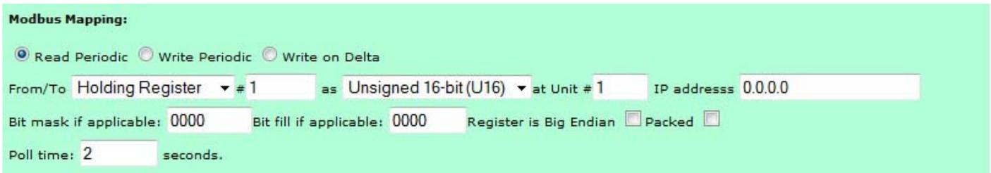
The screenshot shows the 'Modbus Mapping' section with a light blue background. It features three radio buttons: 'Read Periodic' (selected), 'Write Periodic', and 'Write on Delta'. Below these are several input fields: 'From/To' (Holding Register), '# 1', 'as' (Unsigned 16-bit (U16)), 'at Unit # 1', 'IP address' (0.0.0.0), 'Bit mask if applicable: 0000', 'Bit fill if applicable: 0000', 'Register is Big Endian' (unchecked), 'Packed' (unchecked), and 'Poll time: 2 seconds'.
