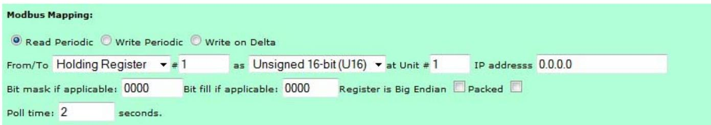
The screenshot shows the "Modbus Mapping:" section with three radio buttons: "Read Periodic" (selected), "Write Periodic", and "Write on Delta". Below are several input fields: "From/To" set to "Holding Register", "# 1", "as" set to "Unsigned 16-bit (U16)", "at Unit # 1", "IP address" set to "0.0.0.0", "Bit mask if applicable:" set to "0000", "Bit fill if applicable:" set to "0000", "Register is Big Endian" (unchecked), "Packed" (unchecked), and "Poll time:" set to "2" seconds.
