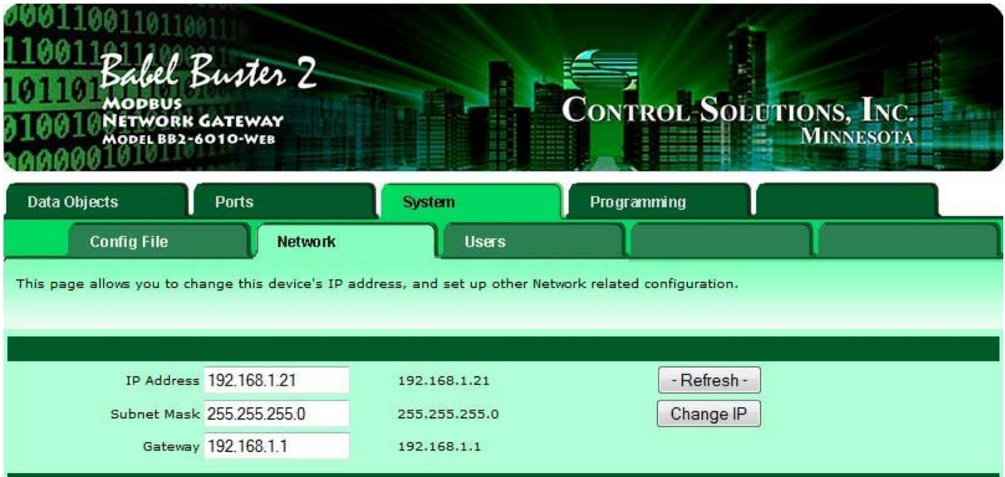
The screenshot displays the web interface for the Babel Buster 2 Modbus Network Gateway. The header features the product name 'Babel Buster 2' and 'CONTROL SOLUTIONS, INC. MINNESOTA'. The navigation menu includes 'Data Objects', 'Ports', 'System', and 'Programming'. Under 'System', the 'Network' tab is selected, showing fields for IP Address (192.168.1.21), Subnet Mask (255.255.255.0), and Gateway (192.168.1.1). A 'Change IP' button is visible.
