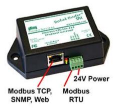
Babel Buster SP: Plug power adapter into power connector marked "Power".
