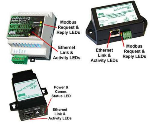
**Babel Buster BB2-6010 and SPX** request/reply LEDs reflect RTU traffic while the Ethernet activity LED will indicate TCP traffic. To see TCP errors, one needs to look at the Errors page in the web UI.
