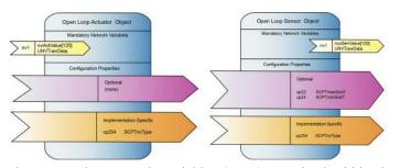
The LonWorks Network Variables (NV's) contained within the Babel Buster gateway are configured as standard sensor and actuator function blocks with user changeable network variable types. Each variable has been allocated the maximum of 31 bytes of memory, meaning any known LonWorks variable type (including UNVTs) can be used. The NV's are bound to other nodes on the LonWorks network using LonMaker or other comparable network management tool.
