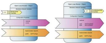
The LonWorks Network Variables (NV's) contained within the Babel Buster gateway are configured as standard sensor and actuator function blocks with user changeable network variable types. Each variable has been allocated the maximum of 31 bytes of memory, meaning any known LonWorks variable type (including UNVTs) can be used. The NV's are bound to other nodes on the LonWorks network using LonMaker or other comparable network management tool.
