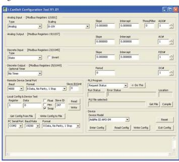
Our PC based configuration tool simplifies setup of analog input type and scaling, analog output scaling, and discrete I/O timing parameters. You can also compile and download your program via this tool.
