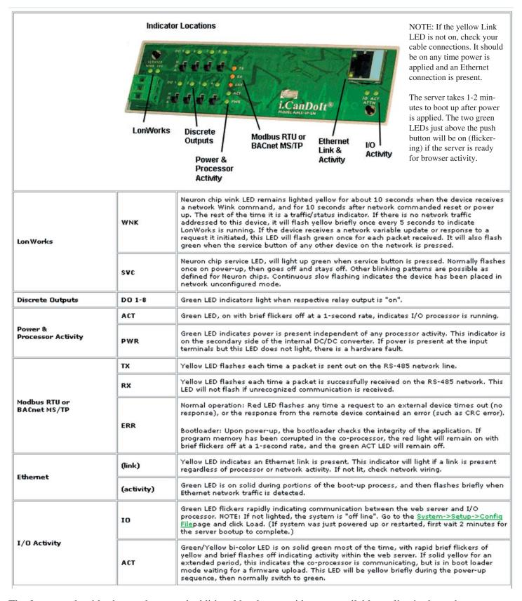
The front panel guide shown above, and additional hardware guides, are available on-line in the web pages served by the device itself. If you do not have access to the device, a demo copy of the device's web site may be found at *www.csimn.com* (after 4/1/2007).
